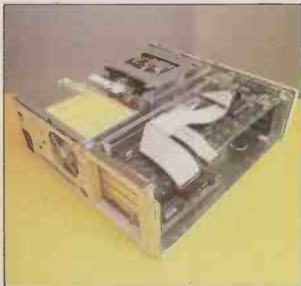
Above: The Sperry Micro IT's expansion cards are laid horizontally to save space. Right: The Sperry is dominated by its VDU.
